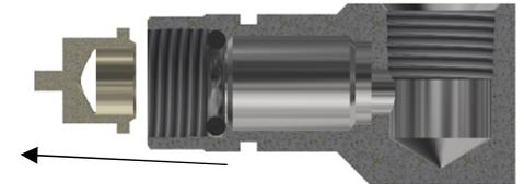
12. Using a pick like tool or flathead screwdriver, remove the O-ring from the groove. Use caution not to scratch the seal groove.
