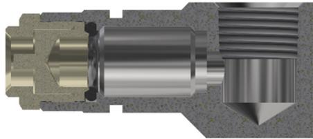
15. Lubricate external O-ring with petroleum jelly and install into external O-ring groove. The KA04CMAT connector utilizes a Teflon ring in this groove in place of an o-ring.
