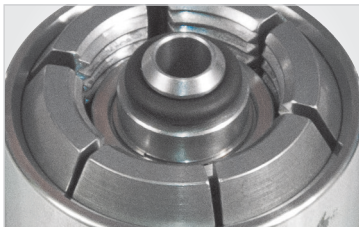
Figure 11. An example of a good O-ring main seal
