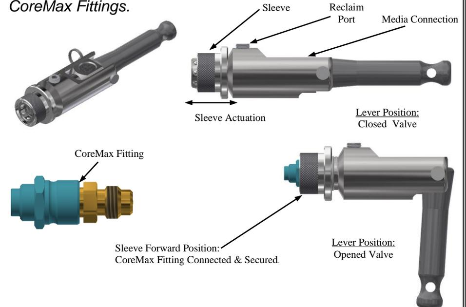
**CMRQD** Connector provides a reliable leak-tight connection that grips and seals a CoreMax Fitting. Simply insert male end of fitting and slide sleeve forward, gripping balls will secure fitting.
