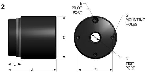
Maximum test pressure: Vacuum to 500 psi
